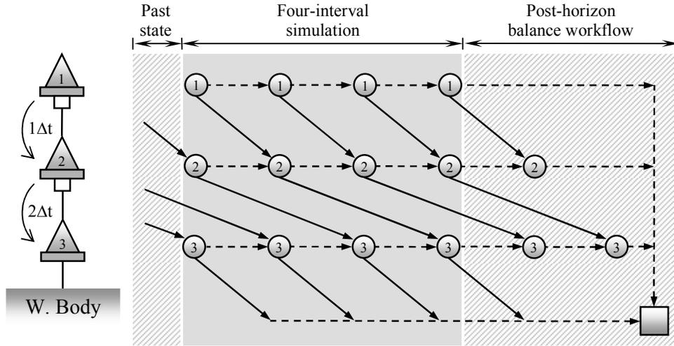
**Figure 6. Three-reservoir and four-interval hydro system as a temporally expanded arborescence with routing effect representation.**
