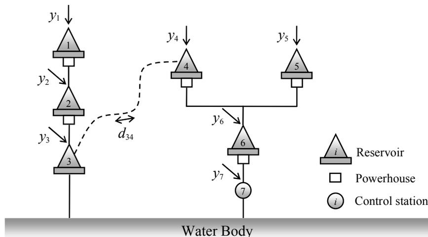
**Figure 5. Hydro elements available for multireservoir simulation.**
