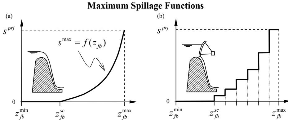
**Figure 4. Uncontrolled and controlled maximum spill functions.**
