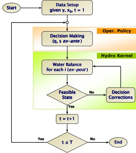
**Figure 8. Simulation algorithm with object-oriented polymorphism applied to partition of operational policy and the hydro computational kernel.**
