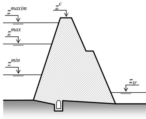
**Figure 1. Reservoir operational water levels.**
