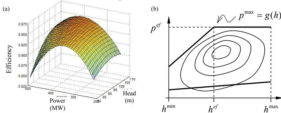
**Figure 3. Example of the turbine efficiency function - hill curve - and maximum and minimum power productions functions.**
