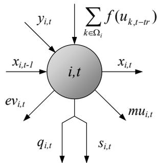
**Figure 7. Mass balance equation equivalence with a network node.**
